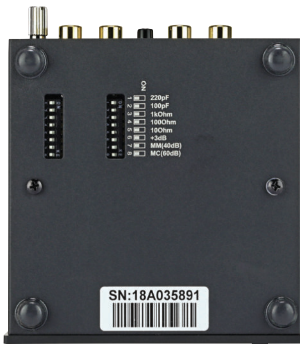
Two rows of recessed DIP switches – one per channel – enable Phono Box S2 Ultra to be ‘matched’ to whatever cartridge (MM or MC) you happen to be using. A tiny screwdriver is needed to flip each switch.
